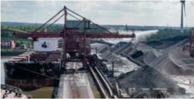
Figure 2. Grab shipunloader at Hansaport, Port of Hamburg, during an autonomous operation.
